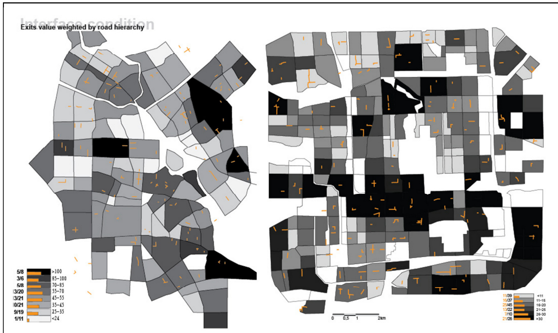
Figure 6 the connectivity of blocks based on the number of exits and network hierarchy in Tianjin (left) and Beijing (right)
